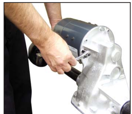
Figure 2 - Remove Mount Bolts
