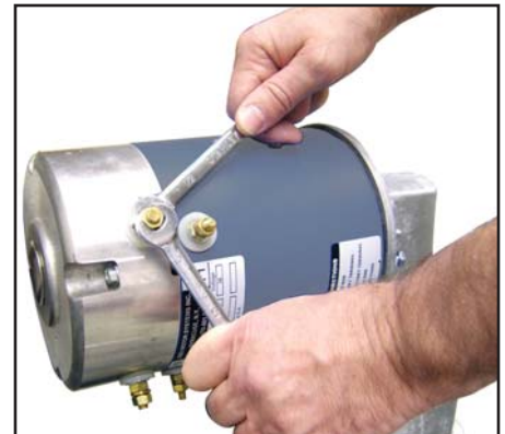
Figure 1 - Double Wrench Technique
